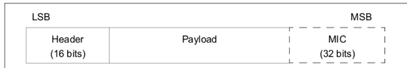
Figure 12: Logical representation of a data channel PDU [BLE-LL, 46]
